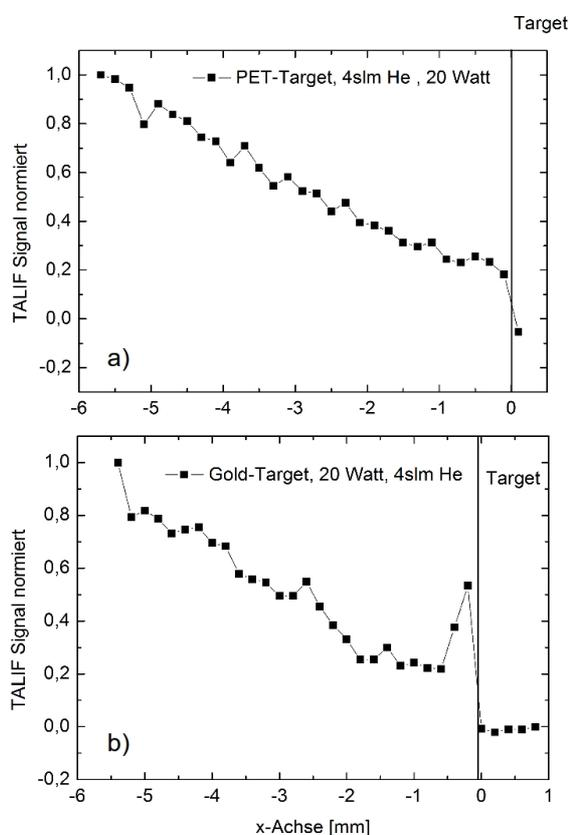
Fig. 1: Oxygen concentration in front of a) a PET and b) a gold substrate
