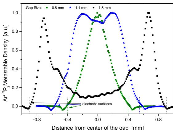
Fig. 1. Ar\* ( $^3P_2$ ) metastable density profiles between the electrodes for 1.8 mm, 1.1 mm and 0.8 mm electrode distance.
